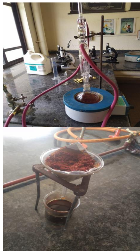
Figure No. 02 Extraction and filter Assembly of Delonix Regia Petals.
